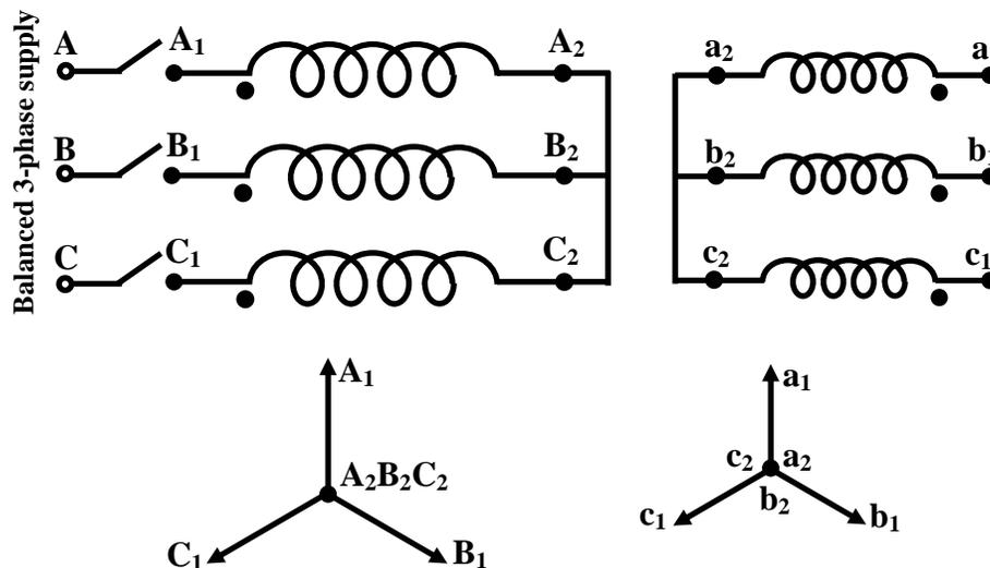
**Figure 26.3: Both primary & secondary are star connected.**
