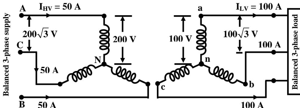
Figure 26.7: Simplified way of showing star-star connection
