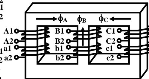
Figure 26.17: A practical core type three phase transformer.
