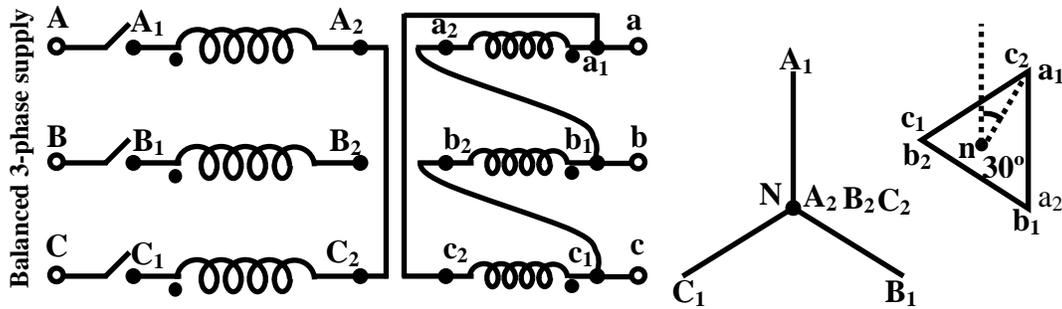
Figure 26.19: Connection and phasor diagram for  $Y d_{11}$ .
