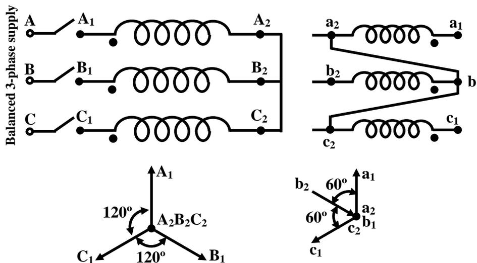
Figure 26.4: Both primary & secondary are star connected.
